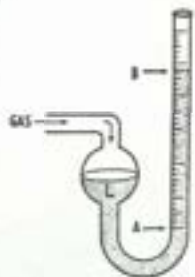
Open-air Manometer (def. 1). Pressure of gas, which enters tube at left, on liquid L, is measured by height of column AB.
